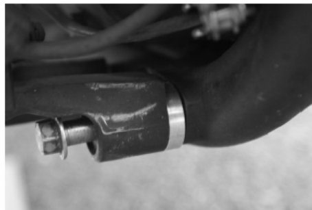
Fig. 2 – Floorboard Mount Spacer Installed
