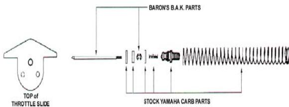
6. Reinstall the vacuum slide along with the diaphragm spring and reattach the diaphragm cover. Verify the slides maintain their full range of movement and do not bind.
