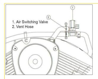
8. Plug connector back into temp sensor and insert remaining vent hose into the BAK backing plate. Be sure to use all the stock hose clamps.
