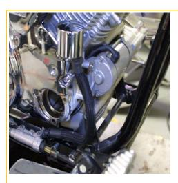
7. Install the new oil relocation assembly by sliding the diverter between the down tubes of the frame and the front of the engine taking care to protect the part from contacting the frame or motor as seen:
