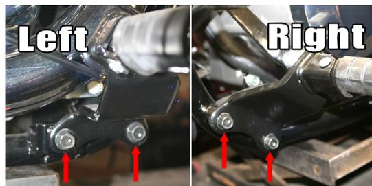
3. At this point, it is best to have someone help you hold the engine guard while you install the hardware. Fish the engine guard carefully through the opening between the front wheel and the frame. Then rotate the guard up into place from the bottom to the top.
