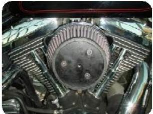
5. Lastly, place the chrome screen into the xXx cover and install over the air filter using the supplied polished flat head bolt and Loctite. Tighten the bolt, clean off the cover and around the air cleaner assembly. Installation is complete. Be sure to clean and re-oil yair filter on a regular basis. Also, be sure to re-torque bolts after riding to ensure air cleaner assembly remains secure.
