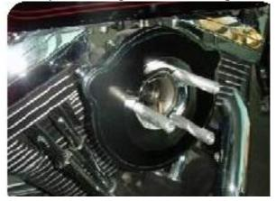
4. Next install the seal plate that fits into the backing plate, sealing off the air/oil channels from the breather bolts. Place filter over seal plate and install black cinch plate with supplied black flat head bolts sealing the air filter and seal plate to the backing plate. To help with orientation, there is a small divot machined into the black cinch plate indicating the top center position. Be sure to apply Locktite to the three flat head bolts. Tighten the bolts to 50 in/lbs of torque.
