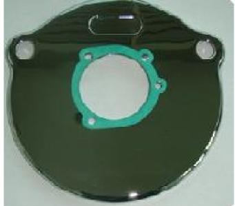
2. Mount the large chrome backing plate to the cylinder heads via the supplied chrome spacers and breather bolts. Spacers have a lip that helps them seat flush in the backing plate. Be sure to use Loctite when securing the bolts. For Evo engines use the larger 1/2-13 breather bolts. For twin cam engines, use the 3/8-16 breather
