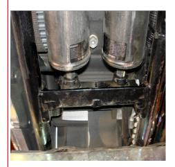
5. Assemble the new shock front hardware (bushing, cup washer and new lowering nut shown below). Use thread locker and install the shocks front hardware using a 3/4" wrench. Do not over tighten.
