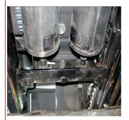
4. Attach a split collar on the shaft of each shock behind the rear bushing cup washer. Use a 9/64'' Hex Allen Key and a dab of blue thread locker on the collar bolts. Do not over tighten.
